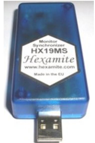
Above on the left is a hx19ms-RS232 version. The RF communication is controlled using a RS232 or a TTL input. HX19MS-USB on the right enable access to the HX19 RF network via USB port. Hexamite provides a visual basic programs with source code to help the programmer understand the communication procedure. The hx19ms understands a few direct commands, its general address type is M.
