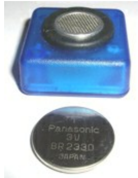
HX19TX Ultrasonic RF battery tag
